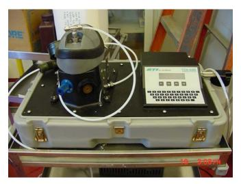
Picture 2: Leak detector Model TDA-99M
