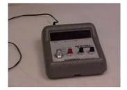
3.1.2. Electric timer, calibrated to hundredths of a minute (Precision Scientific Co.) or equivalent
