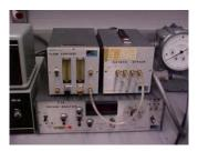
3.1.9. Applied Electrochemistry Oxygen Analyzer - Model S-3A or equivalent.
