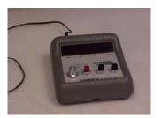
3.1.2. Electric timer, calibrated to hundredths of a minute (Precision Scientific Company) or equivalent.
