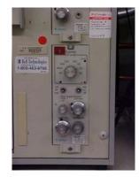
3.1.6. Two channel thermal tip recording system (Gould Model No. RS3200) with carrier amplifier (Model No. 13-4615-35) or equivalent.
