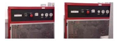
3.1.3. Source of high pressure air. Ingersoll Rand breathing air compressor (5500 psig)- Model BAP20tv3 equipped with a vertical purifier system, capable of delivering 0-5200 psig, a minimum of 1125 psig or equivalent.
