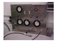
3.1.2. High Pressure Test Stand. A test stand incorporating four Weksler calibrated pressure gauges (two 0-10,000 psig and two 0-3,000 psig) or equivalent.
