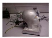
3.1.3. ISI Anthropometric Test heads with tube for measuring breathing resistance and air flows - Model SR-085 or equivalent.
