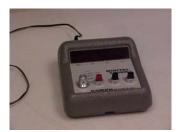
3.1.5. Electric Timer, calibrated to hundredths of a minute (Precision Scientific Company) or equivalent.
