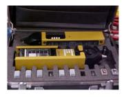
3.1.1. General Radio Noise Dosimeter - Model GR1954 or equivalent.
