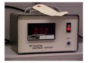
3.1.1. Teledyne Hastings - Raydist Mass Flow Meter - Model NAHL-25 or equivalent.
