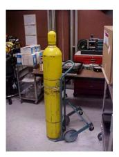
3.1.7. A 300 cubic foot gas cylinder of compressed Grade D air or equivalent.
