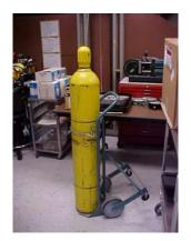
3.1.1. A 300 cubic foot gas cylinder of compressed Grade D air or equivalent.
