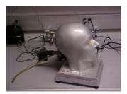
3.1.5. ISI Anthropometric Test heads with tube for measuring breathing resistance and air flows - Model SR-085 or equivalent.
