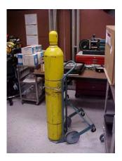
3.1.1. A 300 cubic foot gas cylinder of compressed air or equivalent.
