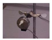
3.1.6. Temperature compensated pressure transducer (Validyne Engineering Model No. DP45) or equivalent.
