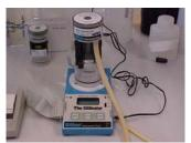
3.1.8. "The Gilbrator", Primary Standard Airflow Calibrator, or equivalent.
