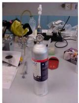
3.1.4. Nitrogen dioxide certified gas cylinder, 1 ppm NO<sub>2</sub>, balance gas helium with 3510-660 regulator.
