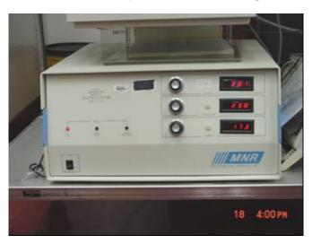
**Picture 5: Flow-Temperature-Humidity Control System**
