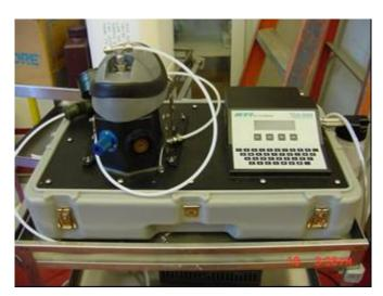
Picture 2: Leak detector Model TDA-99M
