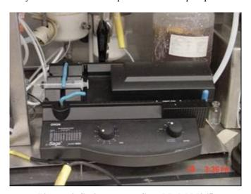
Picture 4: Syringe pump, Sage Model M365
