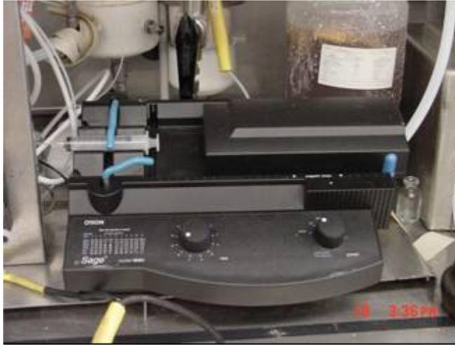
**Picture 4: Syringe pump, Sage Model M365**
