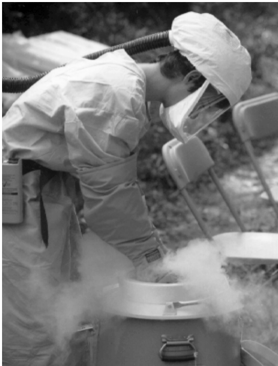
Figure 16. Place field samples on dry ice or in liquid nitrogen until they can be transferred to permanent freezers.
