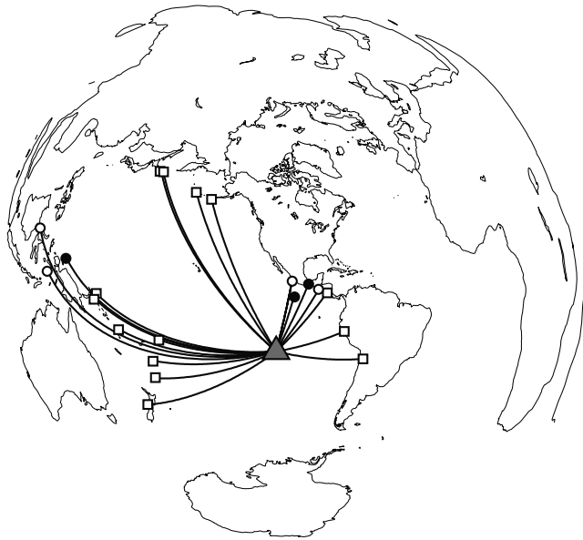
Figure 2. Distribution of events used in the tomographic analysis. Location of MELT experiment shown by triangle. The great circle path between an event and the array is shown by an arcuate line. Symbols at source end of path indicates phase observed from the event: P only (open square), S only (open circle), or both P and S (solid circle).
