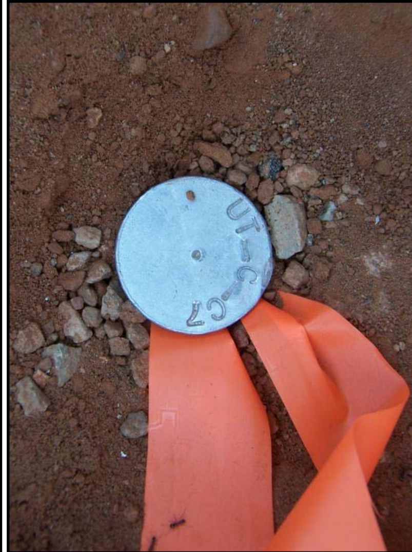
Control point marker
