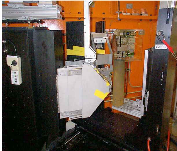
Fig. 5-13. As-cast cylinder liner tube on NRSF2 for stress mapping.
