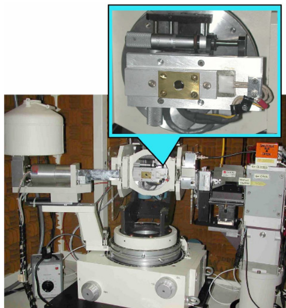
Fig. 5-6. The new elevated-temperature stage (inset) mounted on the 4-axis X-ray goniometer provides new RSUC capabilities for stress and texture measurements at elevated temperature.
