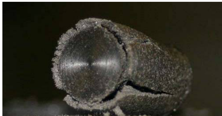
Fig. 3-18. Photograph of bonded test specimen M20979-M after compression testing. Note the core-shell structure.
