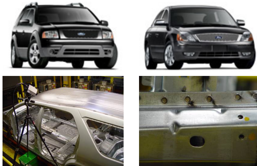
Fig. 6-3. Vehicles produced at the Ford Chicago Assembly Plant. Lower left: laser inspection. Lower right, resistance spot weld inspection.
