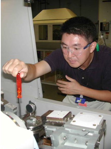
Fig. 5-10. (left) Sangil Han of Georgia Tech, mounting his ring sample to the PANalytical X-ray Diffractometer and (right) retained Austenite as a function of tool flank wear.
