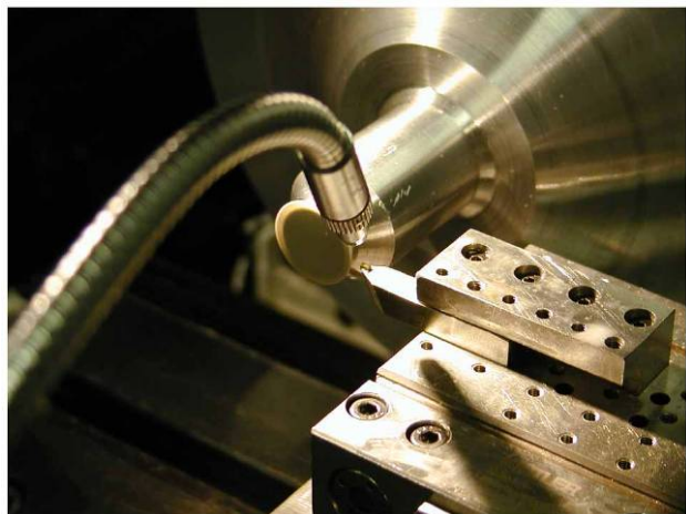
Fig. 2-2. Single-point turning of a silicon nitride disc on the Precitech 2000 DTM.
