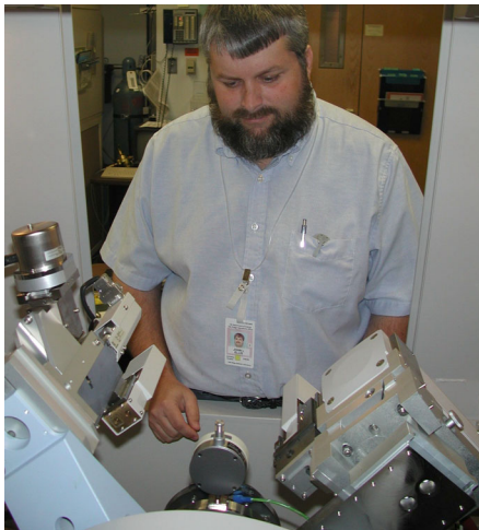
Fig. 5-6. John Ellis setting the sample height (left). The room temperature sin² psi plot shows a large peak shift associated with the compressive residual stress in the alumina scale.
