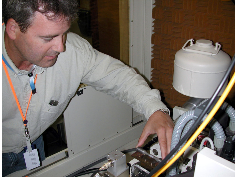
Fig. 5-5. Don Parker, University of Florida-Gainesville, mounting a fatigue specimen on the PTS rotating anode system.
