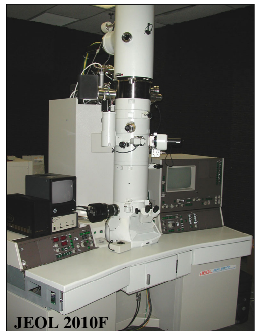
Fig. 1-3. New 2010F provides high-resolution scanning transmission dark-field imaging capability.
