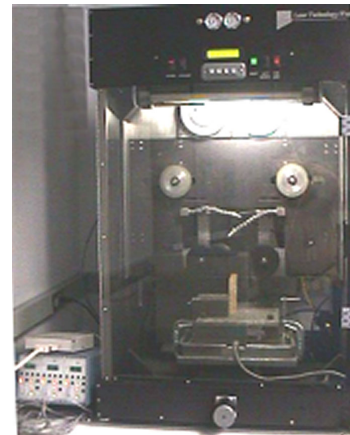
Fig. 2-4. Instrumented diamond wire saw.
