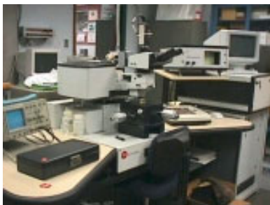
Fig. 2-3. The Ernst Leitz Scanning Acoustic Microscope (ELSAM).
