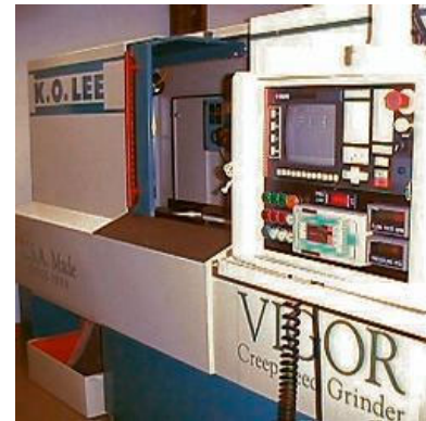
Fig. 2-1. The K.O. Lee instrumented creep-feed grinder.
