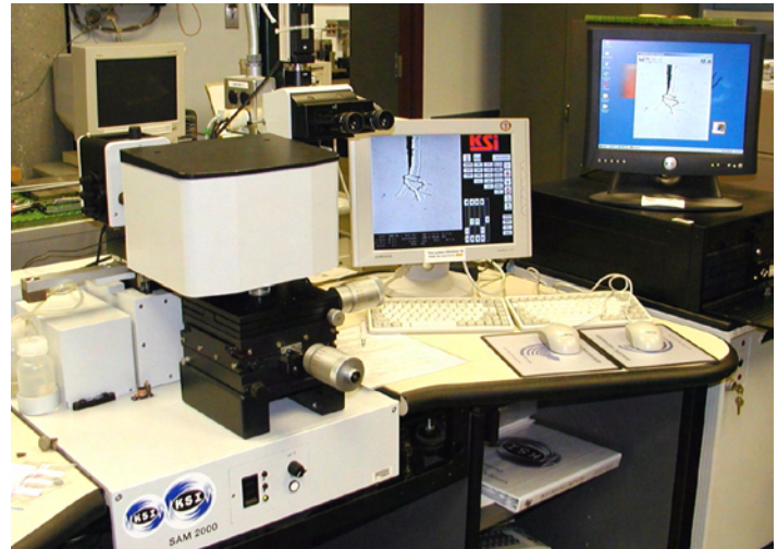
Unique Scanning Acoustic Microscope can probe beneath surfaces for the origins of wear.
