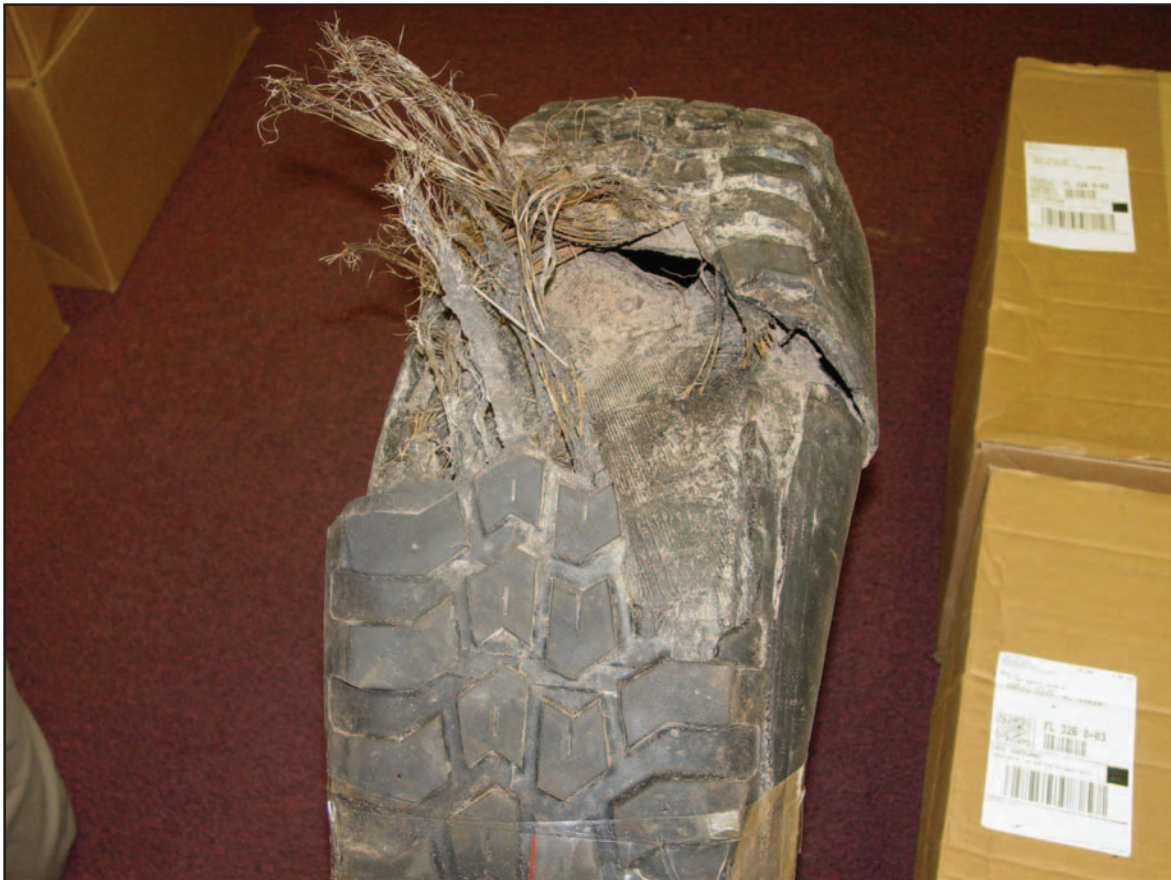
Photo. Right front tire after blow-out
