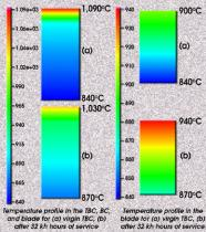
In this example, after 32 kh, degradation of TBC increases blade surface temperature from 900 to 940°C (at constant coolant flow)
