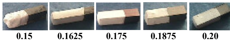
Fig. 5. Resultant coatings from dipping SiC substrates into concentrated mullite suspensions (45 vol%) of varying PEI concentration ranging between 0.15-0.20 mg PEI/m 2 mullite.
