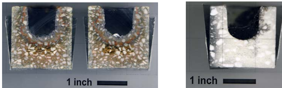
Figure 5 - Large 5 cm “cup” tests samples used to evaluate refractory/slag interactions at 1600°C in an Ar atmosphere. Once exposed, samples are cut in half to show slag penetration. a) slag penetrated refractory microstructure with typical microstructure, and b) improved refractory microstructure.
