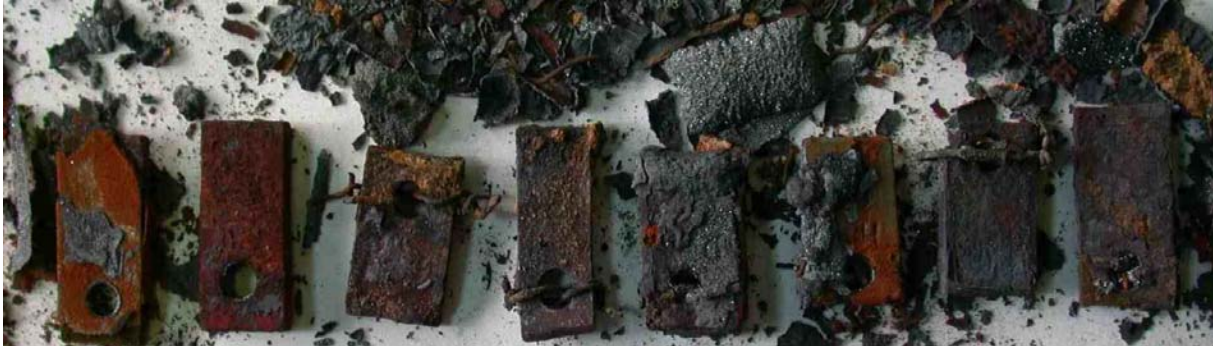
Figure 6. Photograph of duplicate specimens of intermediate-chromium ferritic alloys, that were exposed for 100 h at 650°C to air-1% SO 2 environment containing 300 ppm NaCl.
