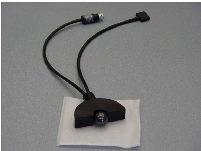
Fig 1. Photograph of first fiber optic array used for laser back scatter experiments. Each fiber is 250 \mu\text{m} in diameter. Shown here is an application for a 25 mm diameter silicon nitride bearing ball. Currently a system is being fabricated with 50 \mu\text{m} diameter fibers.
