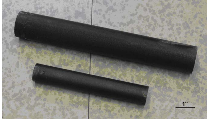
Fig. 10. Pre-oxidized Mo-3 wt% Si-1 wt% B rods scheduled for testing in the Wilsonville, Alabama, coal gasifier.
