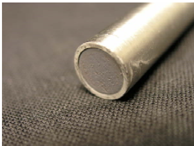
Figure 1: Iron-aluminide microparticle membrane sintered onto a porous Inconel frit press-fit into the end of a 0.95-cm diam. tube
