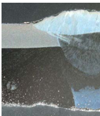
a) Weld "V" (at 1121 F)
