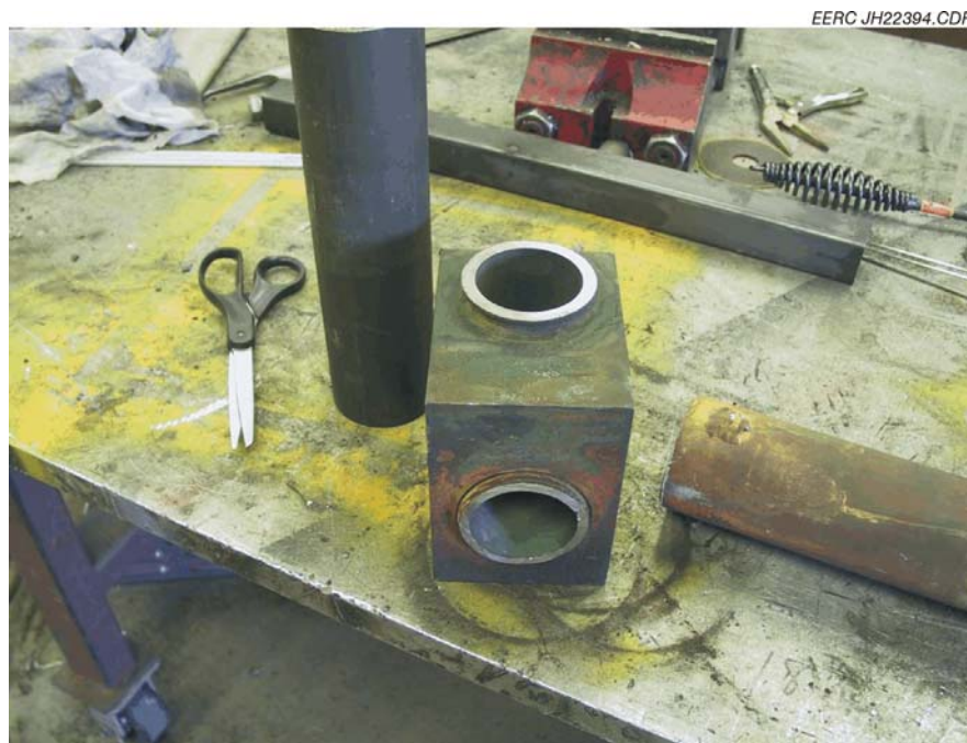
Figure 3. The central MA754 tube and one elbow removed from the HTHX.
