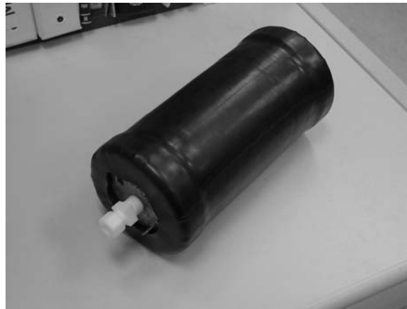
Figure 20 - Experimental ESA cell containing a block of CFCMS material
