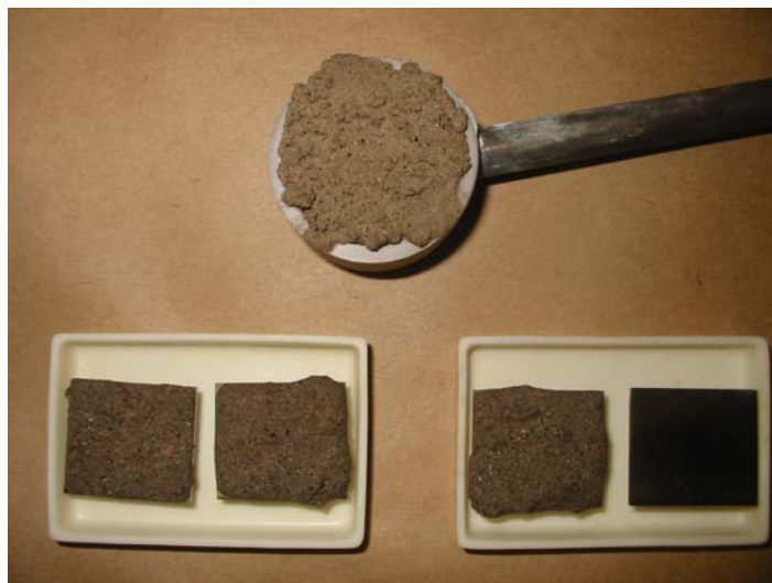
Figure 2 – Electrochemical corrosion rate probe and mass loss coupons prior to testing but after the application of a layer of ash. One coupon (far right) intentionally ash free.
