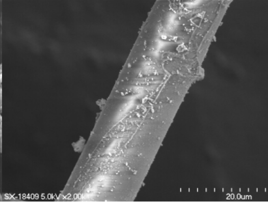
Figure 6. Surface roughness due to faster growth rate
