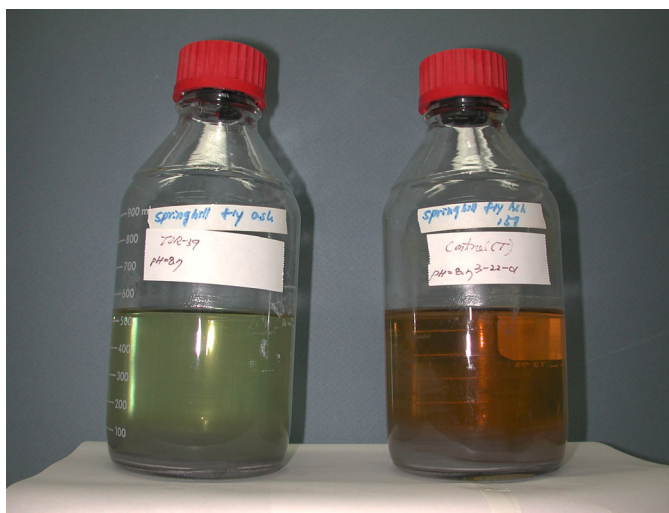
Fig. 1. Scale-up carbon sequestration experiment using Ca-rich fly ash and Fe(III)-reducing bacteria (TOR-35) at 60°C.
