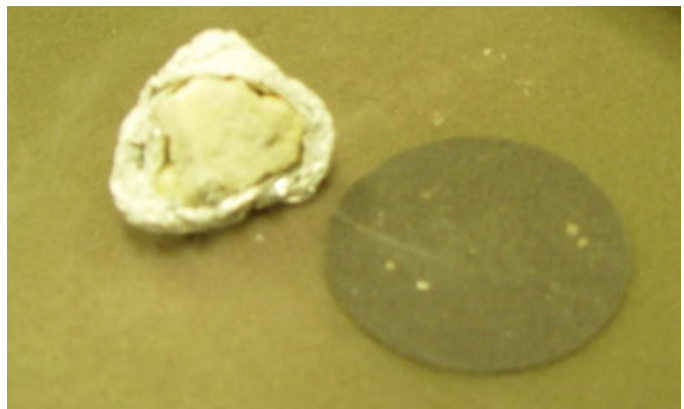
Fig. 6. Preparation of a flat sample for thermal conductivity measurements.
