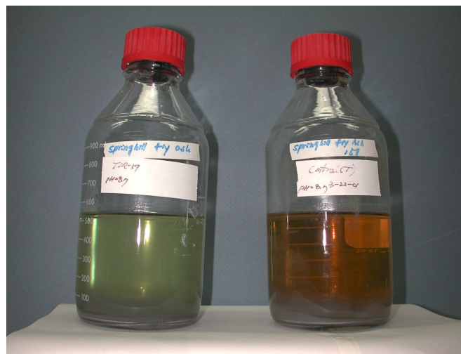
Fig. 6. Scale-up carbon sequestration experiment using Ca-rich fly ash and Fe(III)-reducing bacteria (TOR-35) at 60°C (left 1-L bottle: with bacteria and right 1-L bottle: without bacteria).
