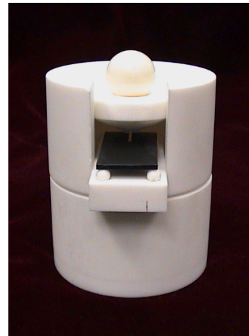
Fig. 3. Picture of high-temperature fixture for the determination of fracture toughness by double-torsion.
