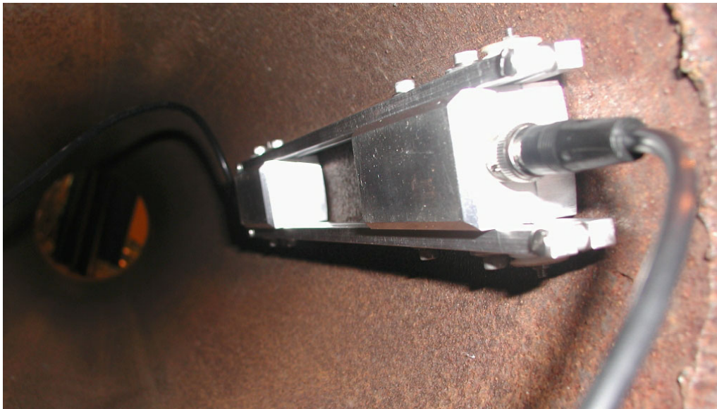
Fig. 2. EMAT configured inside a pipe to detect flaws.
