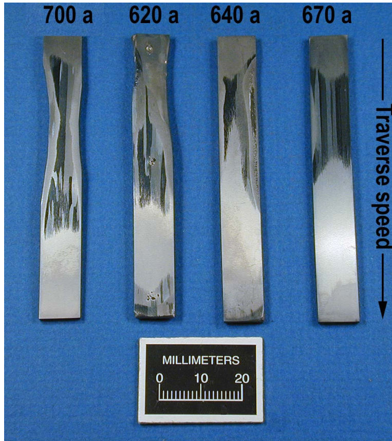
Fig. 11. Etched surfaces of bars of ODS-Fe 3 Al after recrystallization in a moving heat source.
