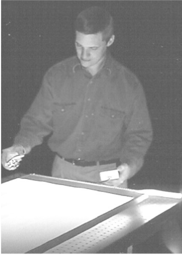
Fiber optic lighting system for lab-scale bioreactor.
