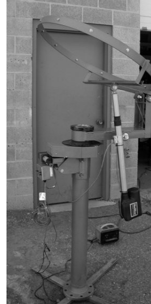
Tracking system for collector.
