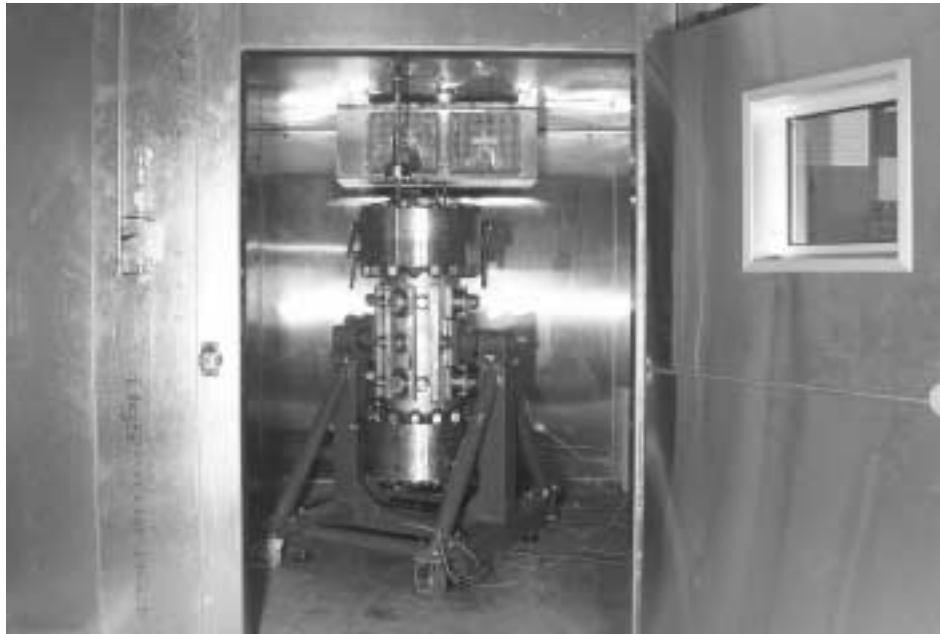
Fig. 1. Photograph of the ORNL Seafloor Process Simulator facility showing the high-pressure vessel and temperature-controlled chamber.
