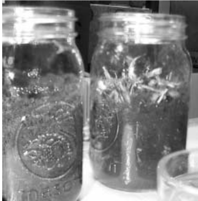
Fig. 2. Experimental units used in soil respiration earthworm/wheat straw factorial experiment. Units were constructed of 400 g dry wt equivalent soil, and depending on treatment, received 8 g chopped wheat straw, and/or 3 adult Eisenia fetida earthworms. Examples shown are landfarm soil without straw (left) and with straw amendment (right), both without earthworms.
