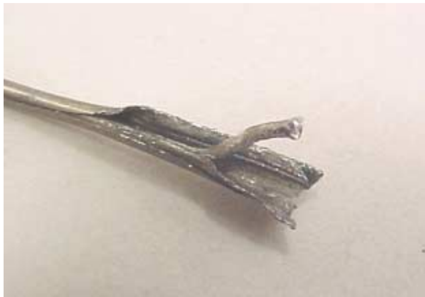
Fig. 2. Construction of Fe-Al composite wire consisting of an Al wire wrapped in an Fe sheath.
