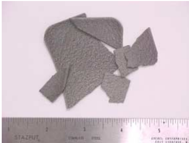
Fig. 3. Photograph wire arc spray coating that spontaneously debonded from its substrate.
