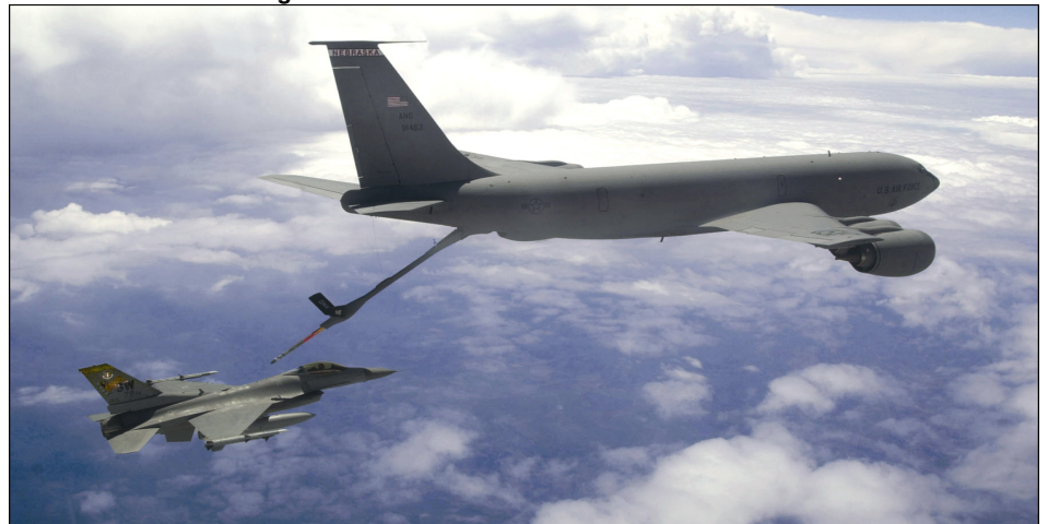
KC-135 Aircraft Refueling an F-16
