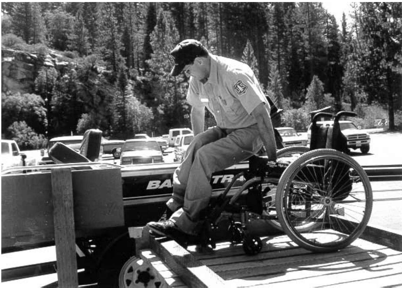
Figure 5 - The boarding platform allows passengers to get into a boat while it is still on land, reducing the risks during loading and unloading.
