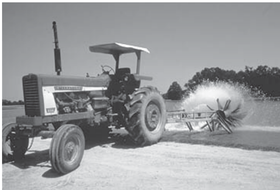
Emergency aerator (PTO)
