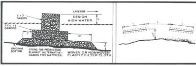
Offshore breakwaters are an acceptable method of shore protection for flat or moderate offshore slopes. The design wave is based on water depth 50 feet lakeward of the structure.
