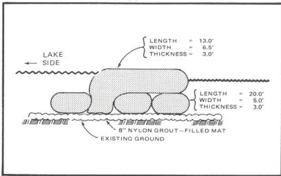
function by reducing the wave energy which strikes the shore and by creating a quiet zone where sand is trapped. The height, length and distance offshore at the breakwater will control the size of the beach which develops behind the structure.
