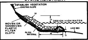
Stone revetment is the preferred method of shore protection. It is economical and suitable for all types of erosion problems when stone available in sufficient size and quantity. The key design considerations, are the dimensions, foundation treatment, and stone size. Construction is not complicated and no special equipment, other than a crane and trucks are needed.
