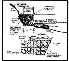
Fence-type structures can be constructed of timber, or metal posts or piling, and wire fence or lumber. The fences can be built of single, double, or triple rows. Posts should be driven below possible scour. Woven-wire fabric is preferred to welded wire fabric.
