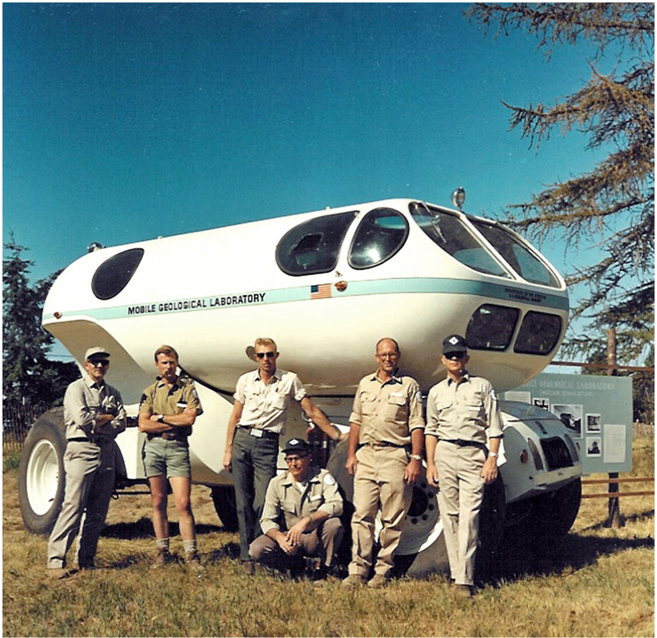
Figure 23-Mobile Laboratory (MOLAB) or Mobile Geologic Laboratory (MGL) designed for NASA by General Motors in 1965 for NASA as a prototype, extended lunar mission vehicle; (a) (l to r) Hal Stephens, Ivo Lucchitta, Bill Tinnin, Bob Sutton and two others (unidentified) standing in front of MOLAB; USGS photo
