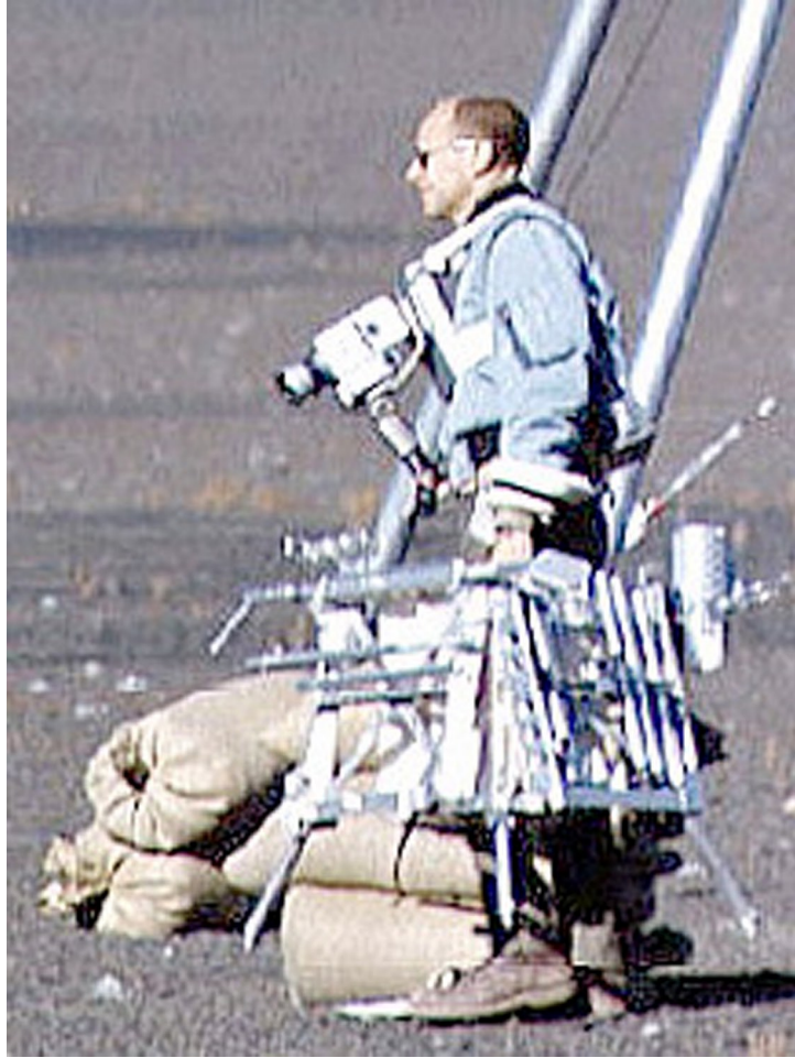
Figure 29-(c) the Apollo 12 Tool Carrier prototype being carried by Apollo 12 astronaut Pete Conrad during field test at Flagstaff in October 1969.
