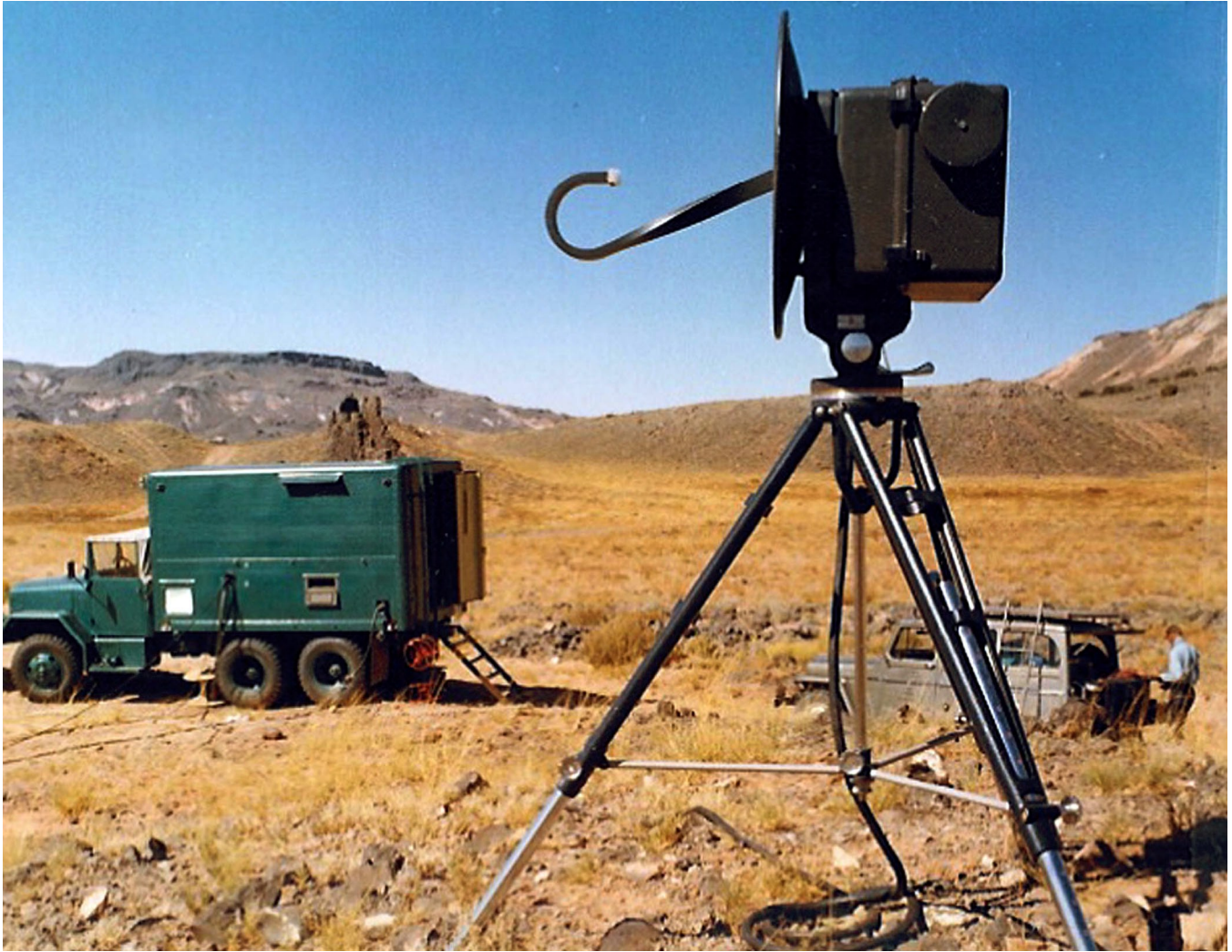
Figure 31-(f) microwave system used to send TV pictures from field to the ADF in the Arizona Bank Building in Flagstaff about 85 miles away; USGS photo P46, F96580c
