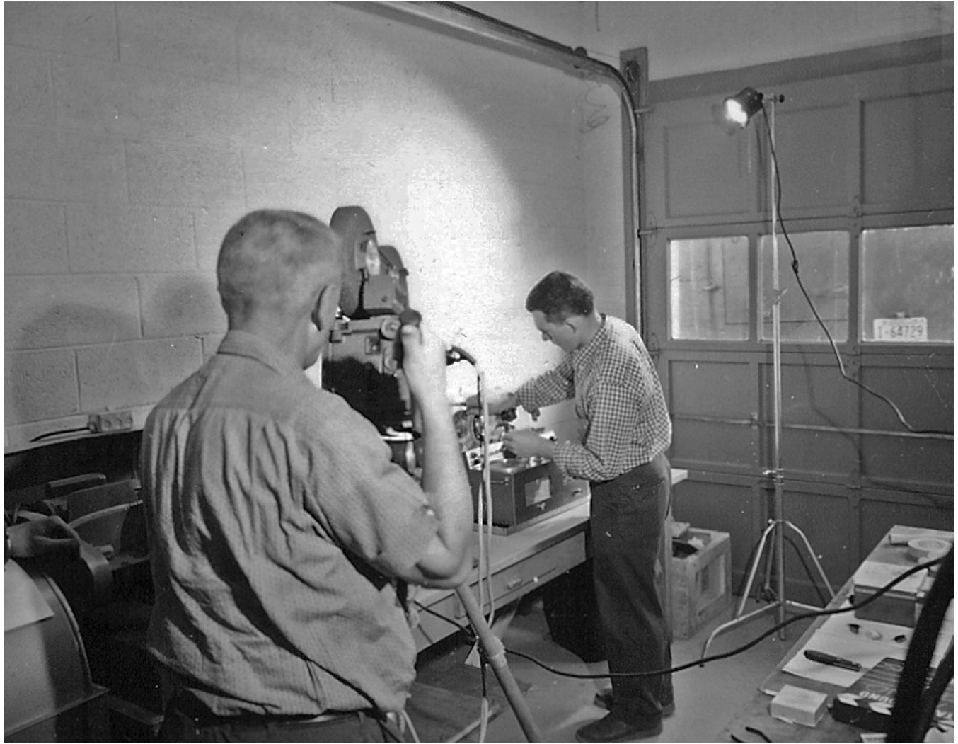
Figure 36 (c) Walt Roeder (Head of the Branch of Astrogeology's Film Documentation Unit) filming George Ulrich making thin sections using semi-automatic thin section machine (see Fig. 34); USGS photo P54, F12652.
