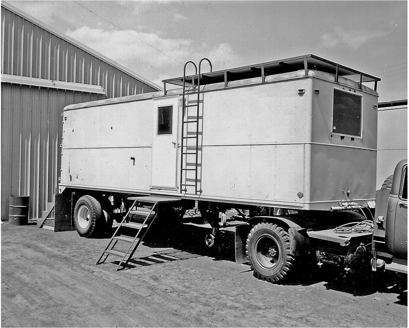
Figure 28-One of several mobile vans (simulating the proposed Houston “science backroom”) that were constructed by the Branch of Astrogeology in Flagstaff to be used during Apollo and Advanced (Apollo Applications Program) geologic field exercises in the mid-1960’s to early 1970’s; (a) outside view of mobile Apollo Data Facility trailer; USGS photo P609 F66894
