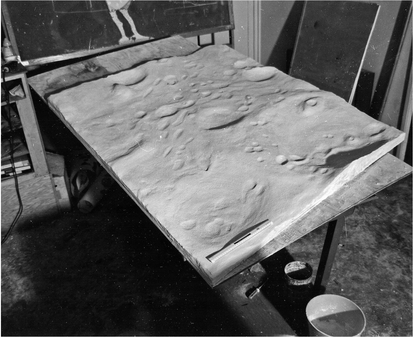
Figure 22-Oblique view of the four-by-six-foot plaster model of the lunar surface constructed by the Branch of Astrogeology following Ranger VII. The topographic relief model was derived from Ranger VII final frame 979; USGS photo.
