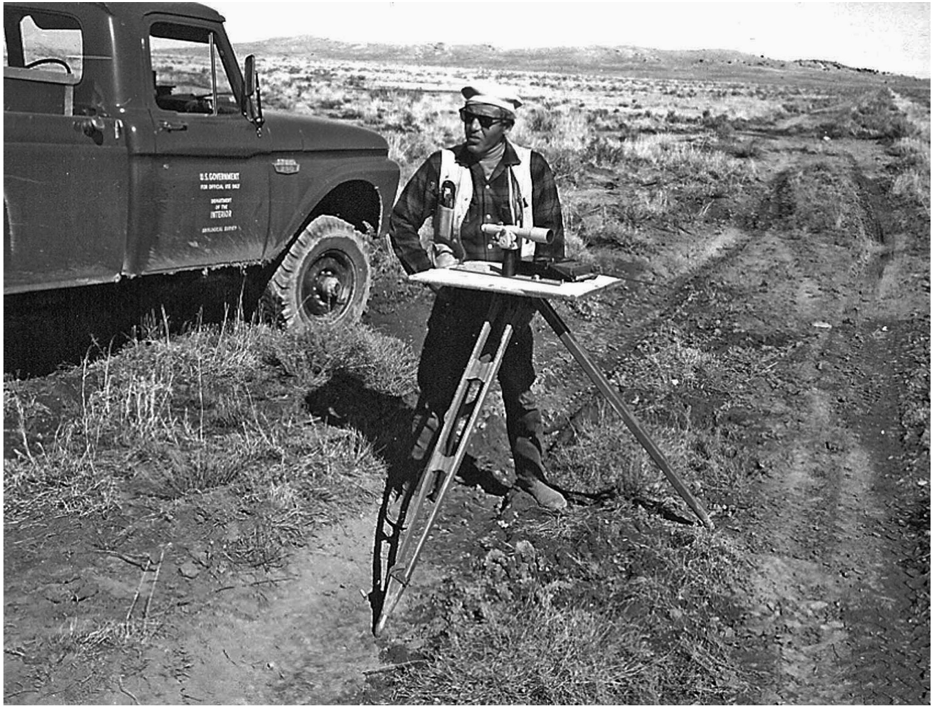
Figure 39-(b) James Crossan, surveyor for the USGS, Branch of Astrogeology (Flagstaff) shown plane-table surveying Trespasser stations during test; USGS photo P82, F33639
