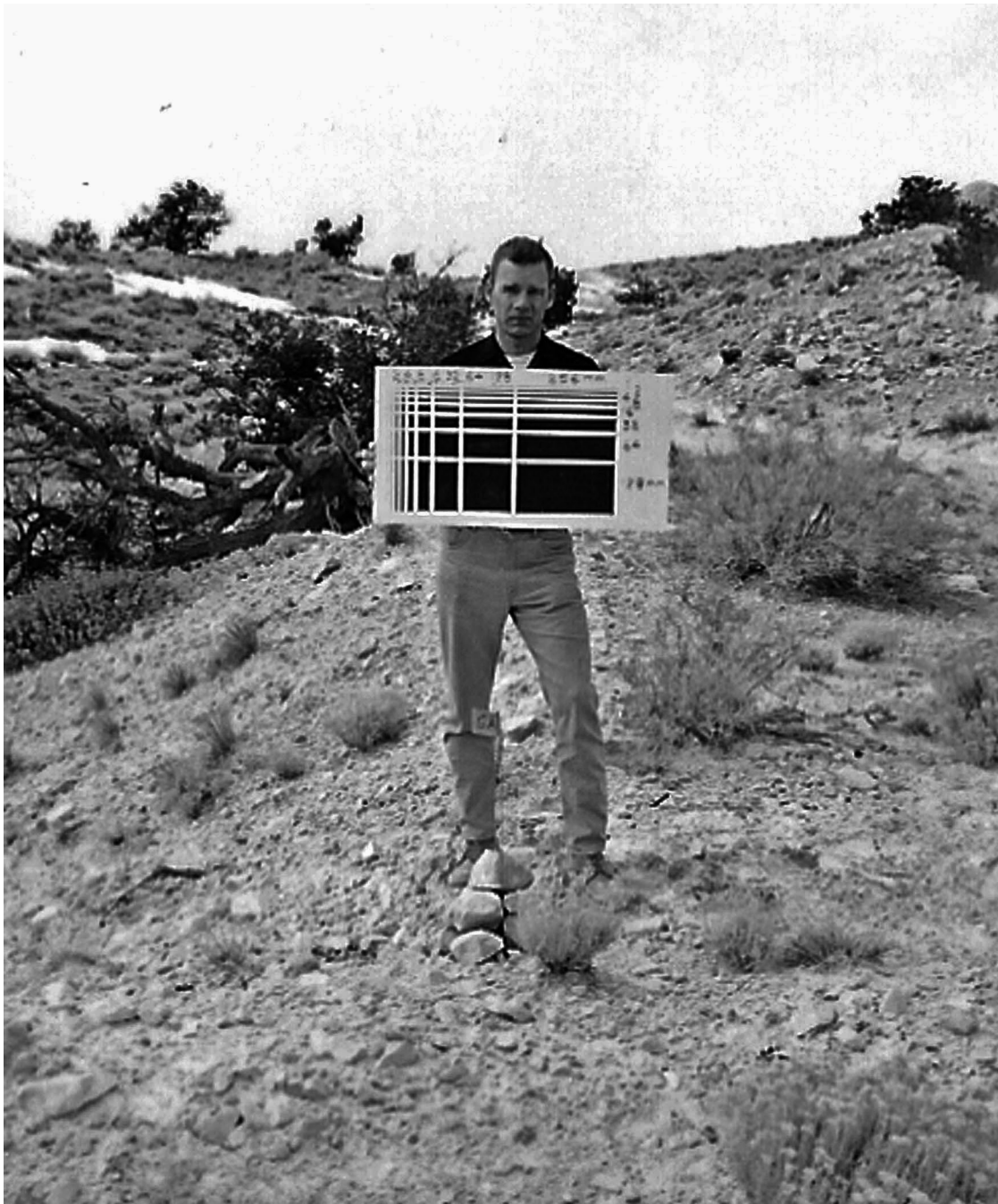
Figure 38-(b) Tim Hait (USGS, Branch of Astrogeology (Flagstaff, Arizona) holding resolution chart during Early Apollo TV camera-resolution test; USGS photo P73, F166115; (c) inside view of the electronics van used during the Early Apollo TV resolution test at Meteor Crater, February 1966; USGS photo P76, F266148; (d) Walt Roeder (left camera), Jim McCord (right camera) and John M'Gonigle from the Branch of Astrogeology's Film Documentation Unit making movie for NASA of Early Apollo TV resolution test at Meteor Crater; USGS photo P73, F266125.
