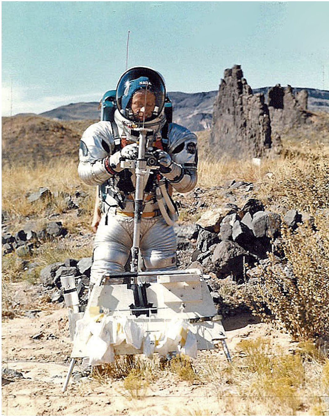
Figure 31-(b) Gordon Swann in suit holding Apollo Lunar Staff prototype; tool carrier in front; USGS photo P45, F96565c
