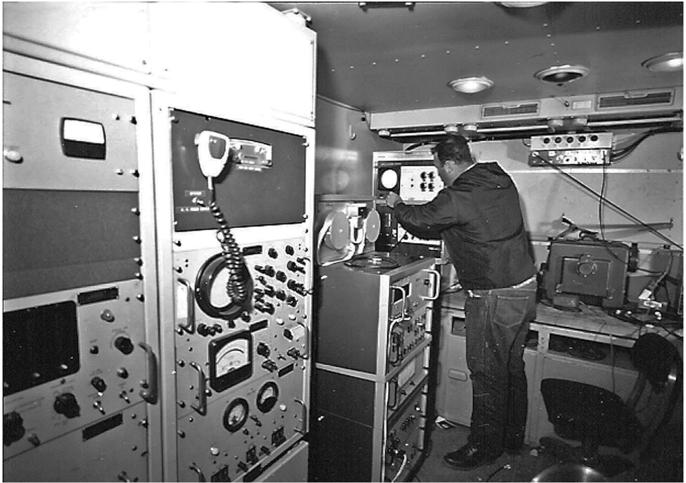
Figure 38-(c) inside view of the electronics van used during the Early Apollo TV resolution test at Meteor Crater, February 1966; USGS photo P76, F266148
