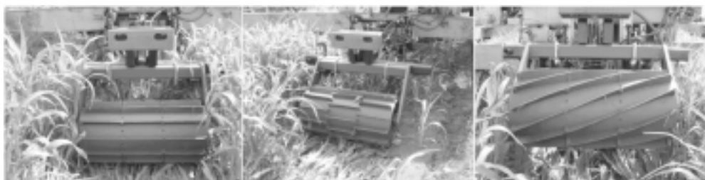
Figure 1. Small roller used for Experiments. On the left is the long-straight blade system, in the center is the short-staggered straight blade system, and to the right is the curved blade system.
