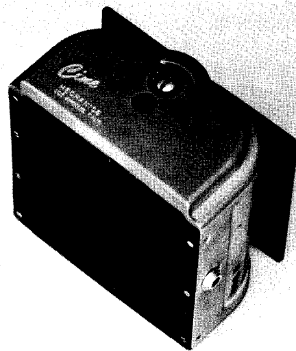
FIGURE 5.—A variation of the device shown in figure 4 was developed for the Gemini program, with a plate attached for storing the magazines. After experimenting with a silver finish, the decision was made to continue with a black finish until the lunar landing.
