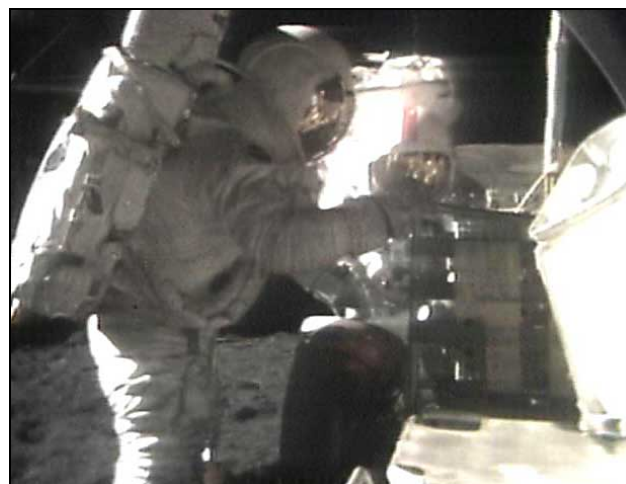
After a misplaced hammer ripped off part of the right rear fender during EVA 1, the crew works to install a jury-rigged extension made from a map and "duct" tape.
