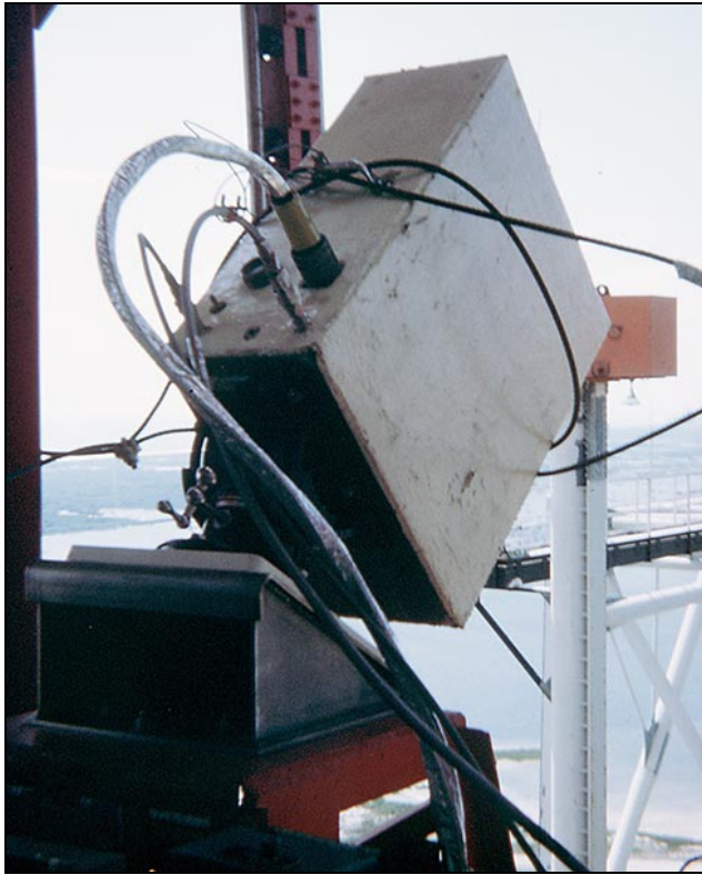
Westinghouse FS Color camera mounted on top of the Apollo 13 Launch Umbilical Tower
