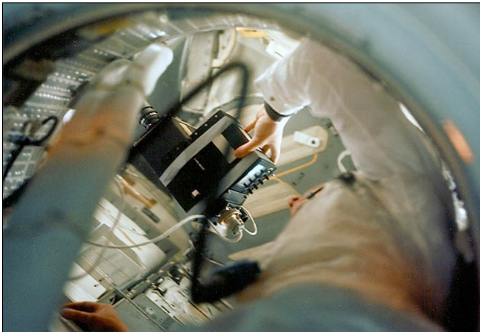
Color TV Camera and Monitor in use by Neil Armstrong inside the LM
