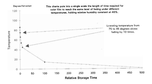
Figure 3: Effect of Temperature on Color Fading (Holding Relative Humidity at 40%) (From proposed *SMPTE RP 131*)
