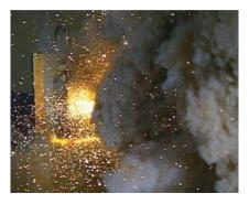
An arc flash is the sudden release of electrical energy through the air when a high-voltage gap exists and there is a breakdown between conductors.
