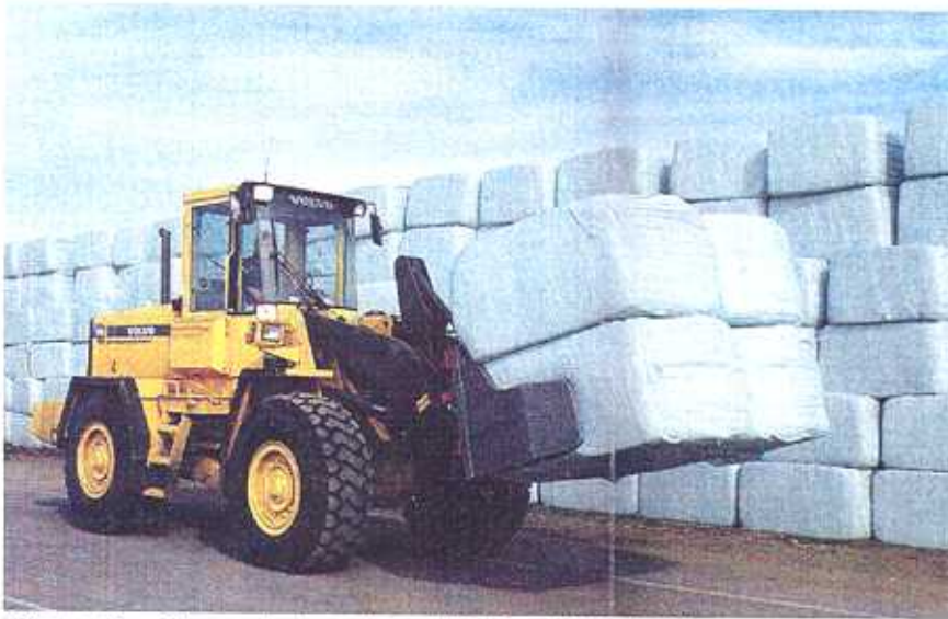
Figure 1. Example tractor with 'grabbing' lift arms for handling bales.
