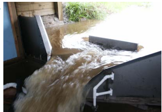
Flood runoff being measured with a dropbox weir in an urbanized watershed after rain storm in August
