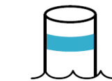
MOORING BUOY WHITE WITH BLUE BAND MAY SHOW WHITE REFLECTOR OR LIGHT
