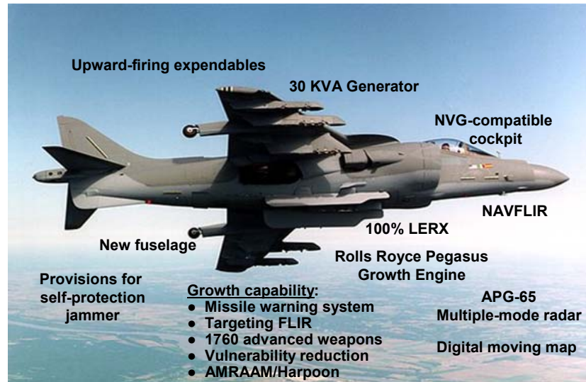
Figure 1. Features of the Remanufactured Harrier II
