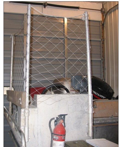
(Above) To protect themselves from jumping carp injury, the project team constructed and anchored a "carp guard" to the boat used for carp research.
