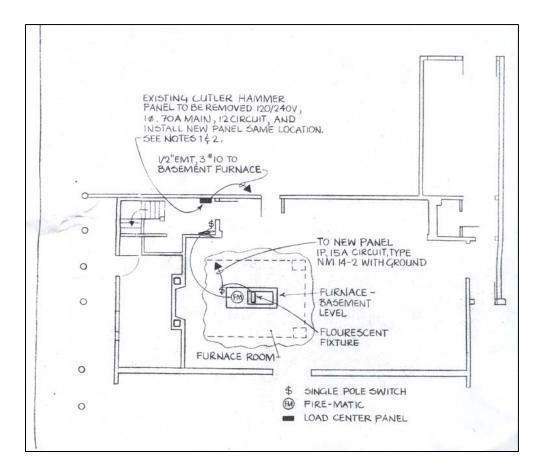
Figure 110. Little Studio, installation of new electrical panel: basement level plan, 1995.
