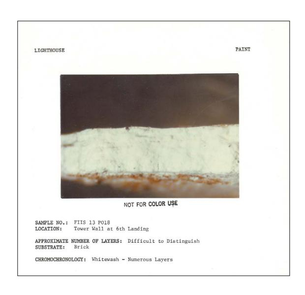
**Figure 107.** Tower interior: paint sample #FIIS 13 P018, wall at sixth landing (1983).
