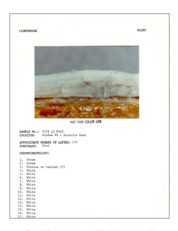
Figure 184. Tower interior: paint sample #FIIS 13 P025, interior sashes (1983).
