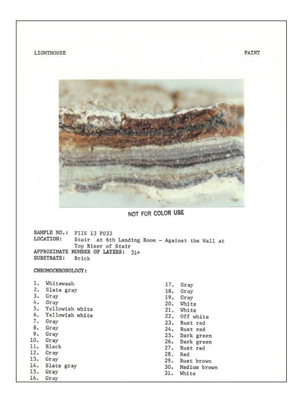
**Figure 141.** Tower interior: paint sample #FIIS 13 P033, wall of sixth-landing room (1983).
