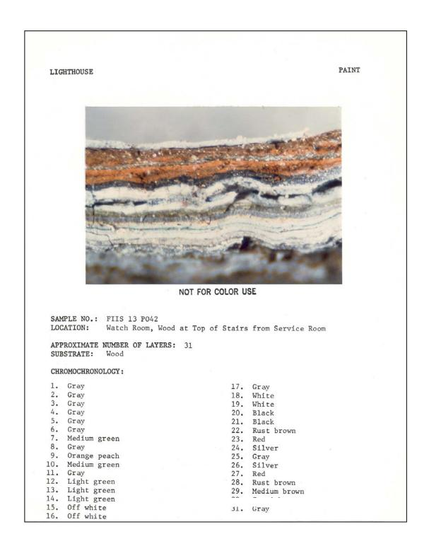
**Figure 119.** Tower interior: paint sample #FIIS 13 P042, wood where Service Room stairway reaches Watch Room (1983).
