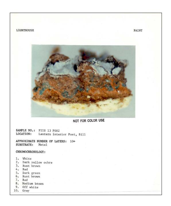
Figure 195. Tower interior: paint sample #FIIS 13 P002, lantern sill (1983).
