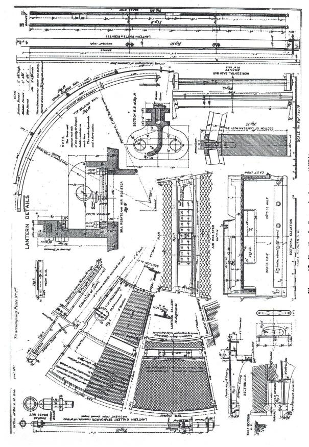
Figure 62. Details of a first-order lantern (1871).
