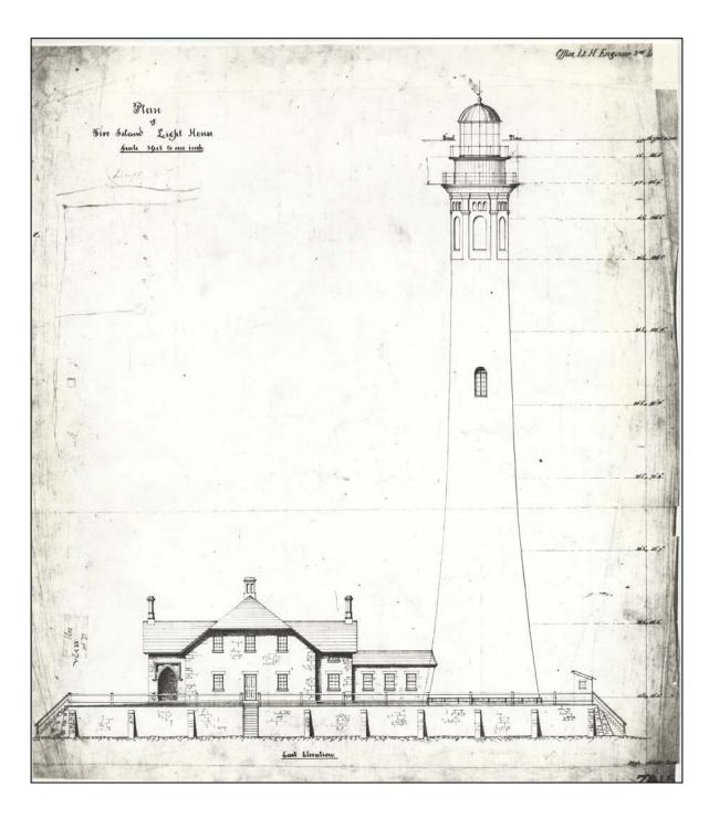
**Figure 6**. Fire Island Lighthouse and Keeper's Dwelling: east elevations, ca. 1857.
