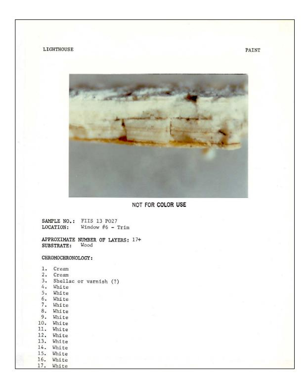
Figure 185. Tower interior: paint sample #FIIS 13 P027, window frame (1983).
