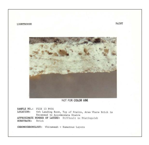
**Figure 109.** Tower interior: paint sample #FIIS 13 P034, sixth-landing room wall, area recessed for stairway (1983).
