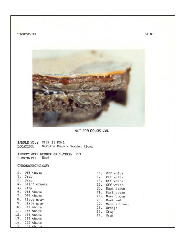
**Figure 117.** Tower interior: paint sample #FIIS 13 P041, wood of Service Room floor (1983).
