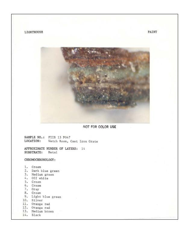
Figure 110. Tower interior: paint sample #FIIS 13 P047, Watch Room vent box (1983).
