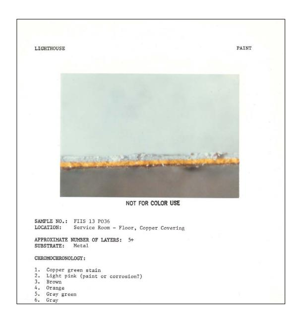
**Figure 116.** Tower interior: paint sample #FIIS 13 P036, copper on Service Room floor (1983).
