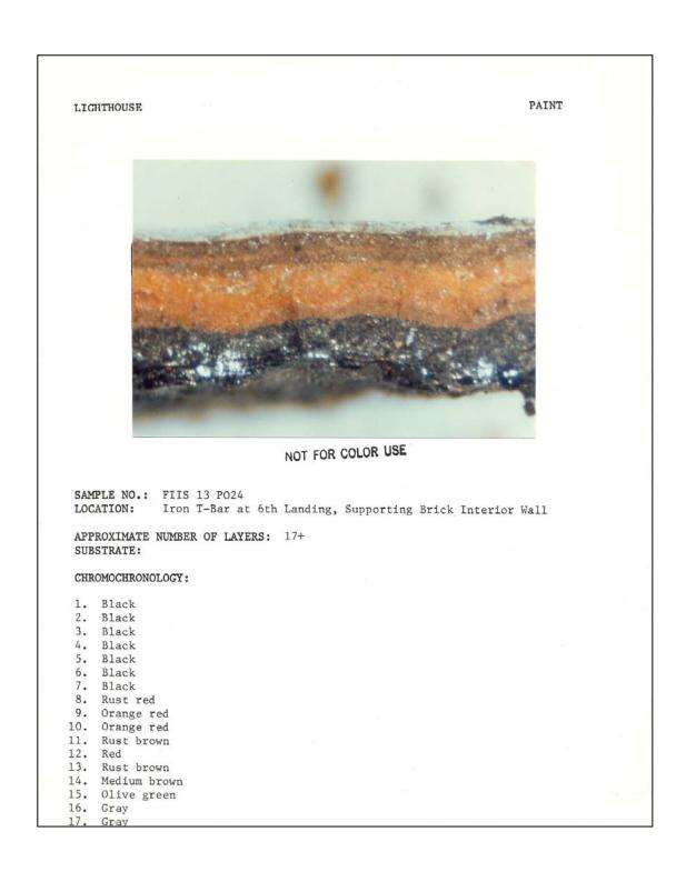
**Figure 108.** Tower interior: paint sample #FIIS 13 P024, iron bar under partition at sixth-landing room (1983).
