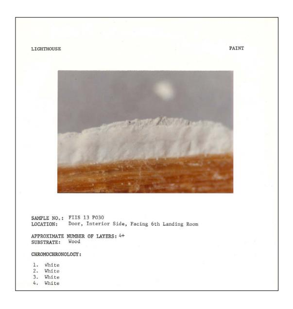
**Figure 167.** Tower interior: paint sample #FIIS 13 P030, room side of sixth-landing room door (1983).
