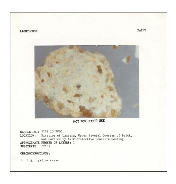
**Figure 91.** Tower exterior: paint sample #FIIS 13 P005, wall not covered by coating (1983).
