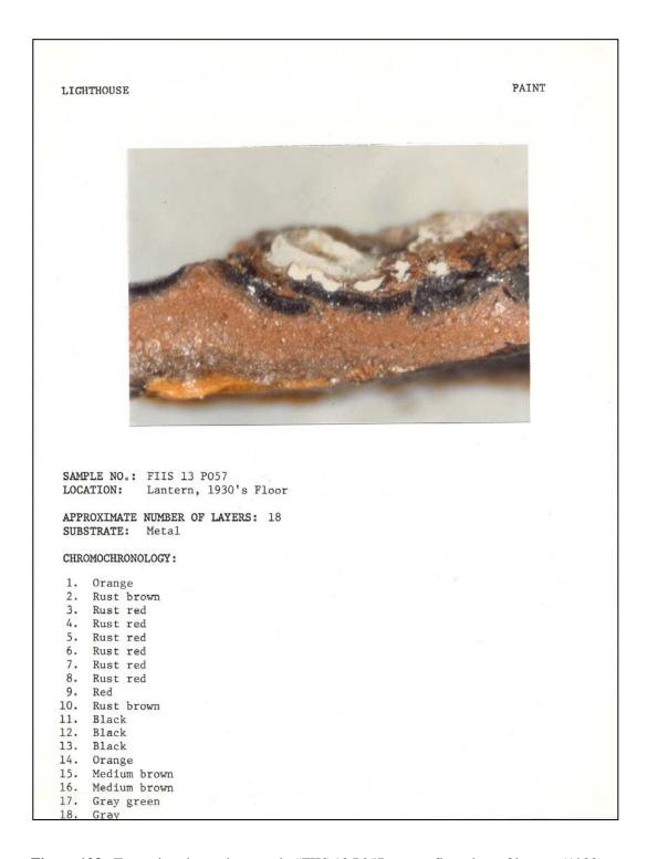
Figure 123. Tower interior: paint sample #FIIS 13 P057, center floorplate of lantern (1983).
