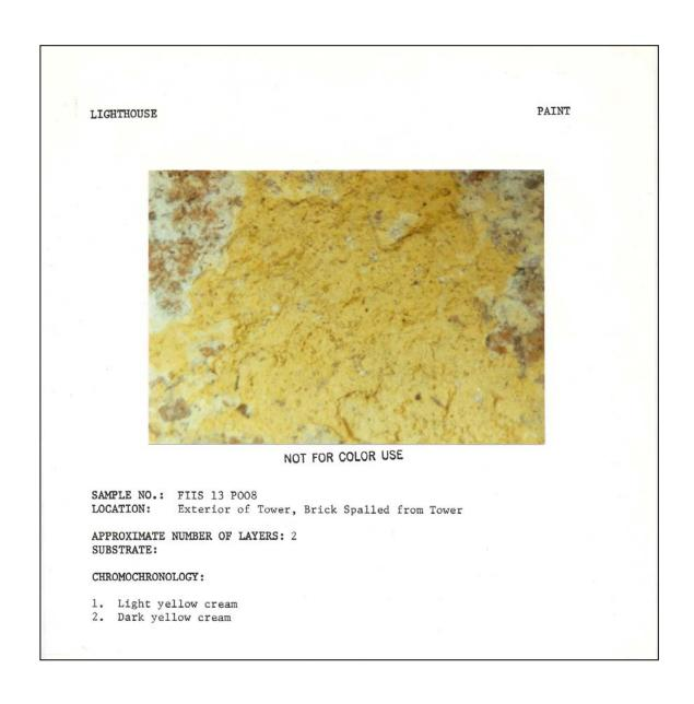
Figure 92. Tower exterior: paint sample #FIIS 13 P008, spalled brick (1983).
