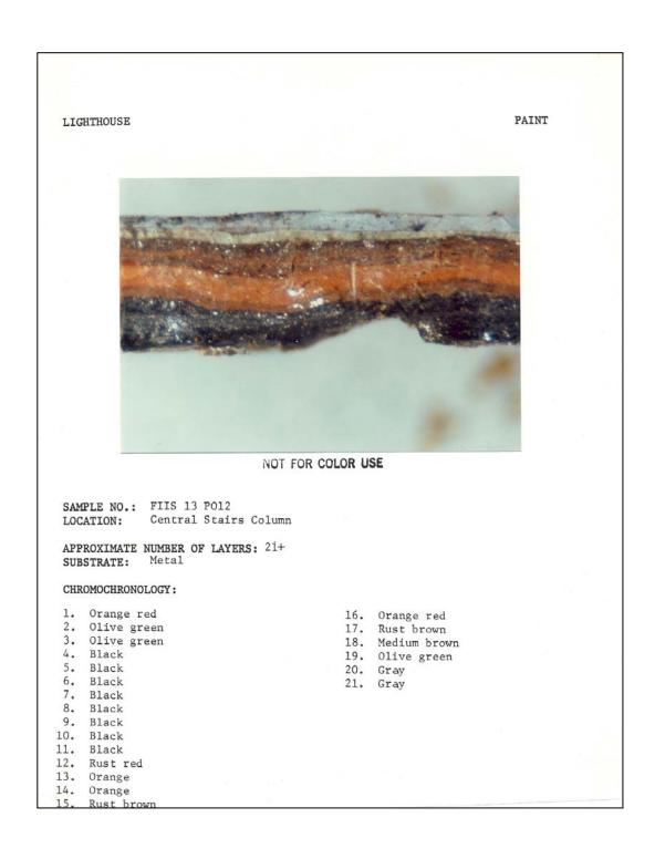
Figure 147. Tower interior: paint sample #FIIS 13 P012, central column (1983).
