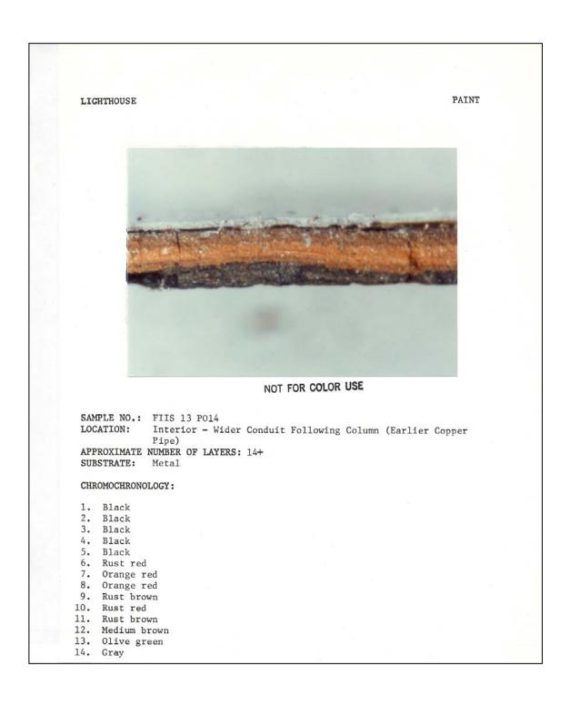
Figure 156. Tower interior: paint sample #FIIS 13 P014, conduit A (1983).
