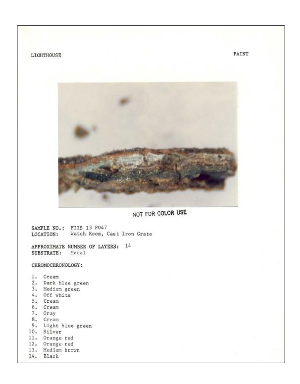
Figure 111. Tower interior: paint sample #FIIS 13 P047, Watch Room vent box (1983).
