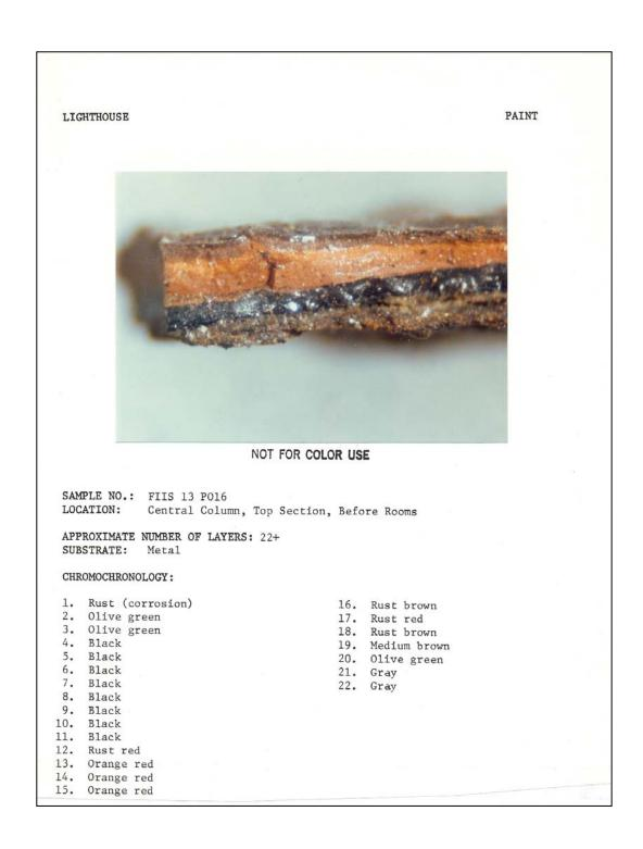
**Figure 148.** Tower interior: paint sample #FIIS 13 P016, central column near sixthlanding room (1983).
