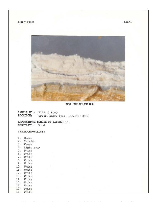
Figure 163. Tower interior: paint sample #FIIS 13 P060, entrance door (1983).
