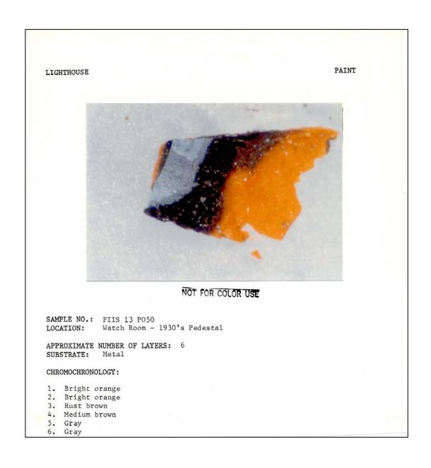
Figure 210. Tower interior: paint sample #FIIS 13 P050, Watch Room pedestal (1983).
