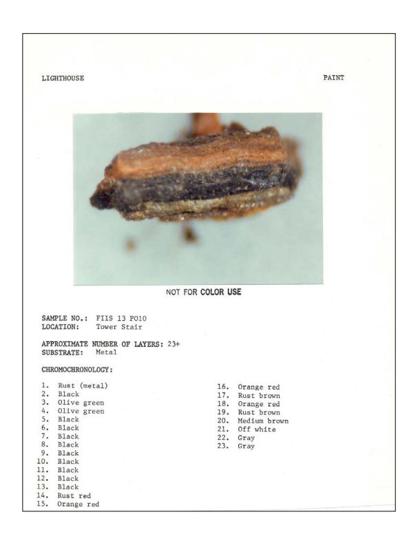
Figure 137. Tower interior: paint sample #FIIS 13 P010, main stairway (1983).
