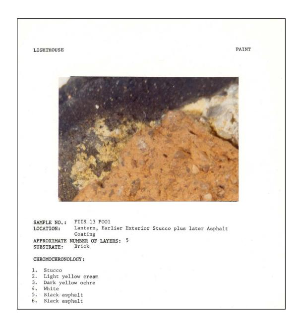
Figure 90. Tower exterior: paint sample FIIS 13 P001, wall covered by coating (1983).
