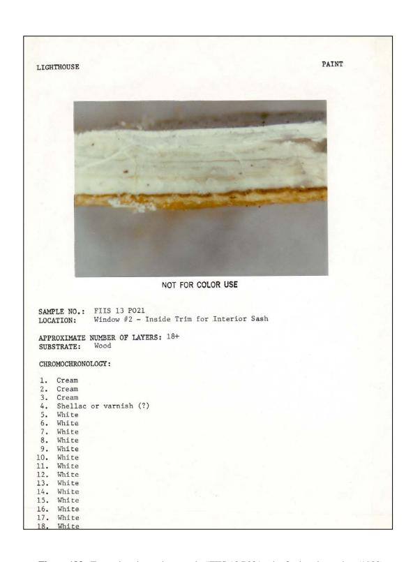
Figure 183. Tower interior: paint sample #FIIS 13 P021, trim for interior sashes (1983).
