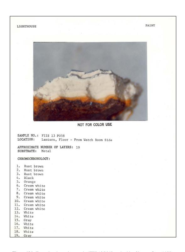
Figure 124. Tower interior: paint sample #FIIS 13 P058, underside of lantern floor (1983).
