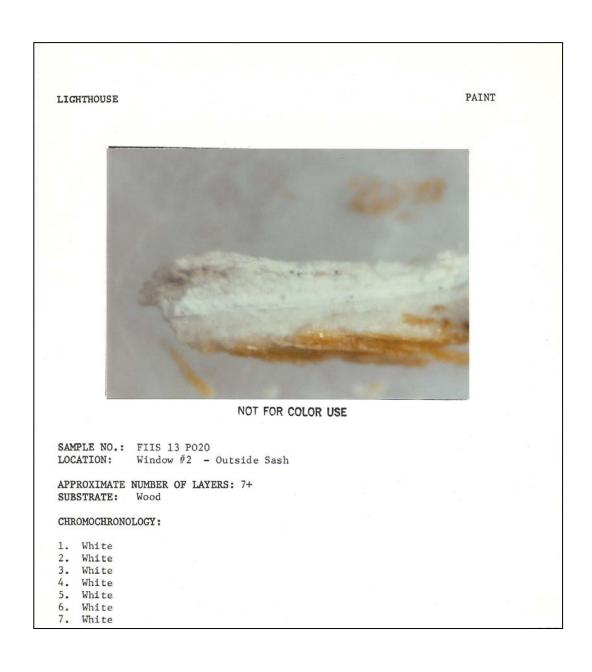
**Figure 182.** Tower exterior: paint sample #FIIS 13 P020, outer side of storm sashes (1983).
