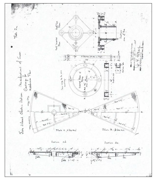
Figure 68. Details of Watch Room floor (1894).
