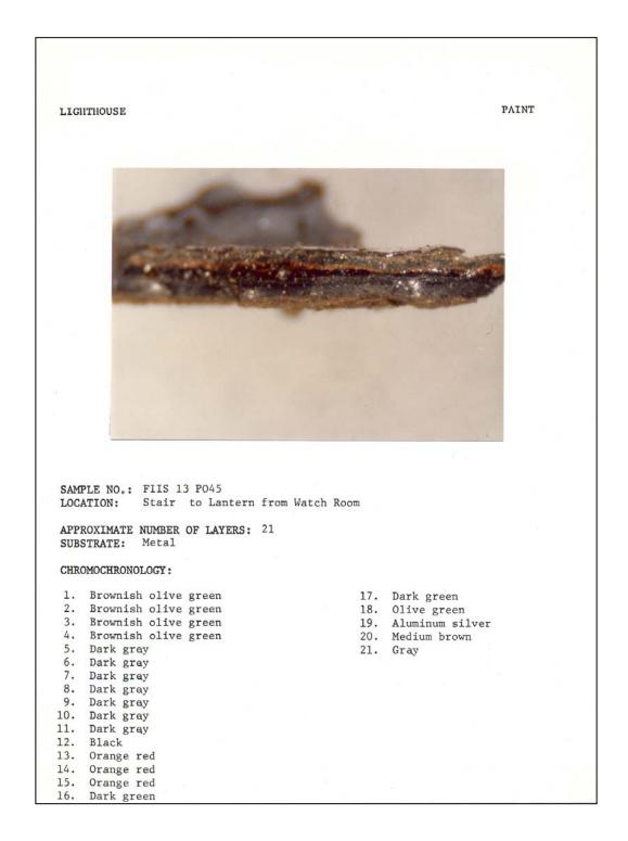
Figure 144. Tower interior: paint sample #FIIS 13 P045, Watch Room stairway (1983).
