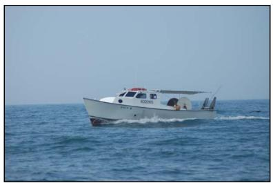
Figure 7.5.2. Fishing Vessel *Lucy B*. with Drop Net Rig. Photo by Danielle Waples.
