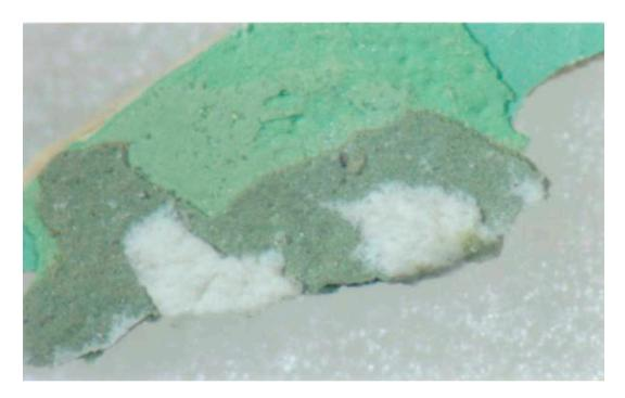
Fig. 14 Paint Sample WRBR-VC-P032 Removed from a Door in the Office Area of the Wright Brothers National Memorial Visitor Center, Showing Original Green-Colored Paint and White-Colored Primer (Viewed at 30x), (2000).
