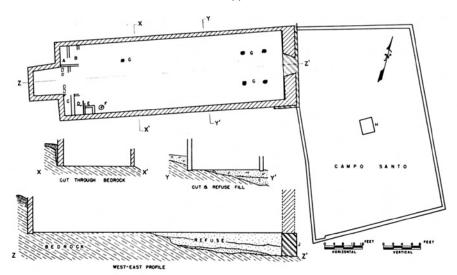
FIGURE 17 The church of San Isidro, plan and sections, and the campo santo. A, C, closetlike enclosures probably serving as sacristies; B, probable side altar; D, wall of raised sanctuary area; E, base for stand or cupboard holding baptismal supplies; F, sacrarium; G, stone bases for upright roof supports; H, masonry base for a cross in the campo santo; J, foundation—it occurs only at the east end of San Isidro.
